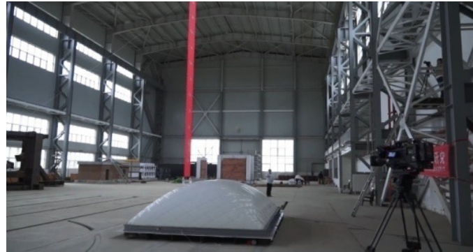
Free-fall hard objects impact experiment
